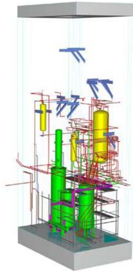
A computerized drawing that depicts the vessels and piping remaining in XC-3 as of late August. The vessels colored in yellow were removed in early September.
