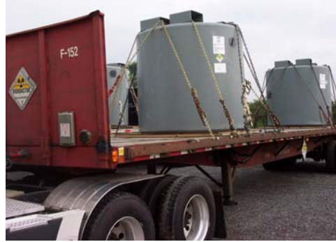
IP-2 containers, like the ones used for shipping sodium-bearing waste in 2004 shown above, will be used for this project
