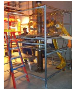
Mock-up of cutting 8-inch ventilation line in glove bag
