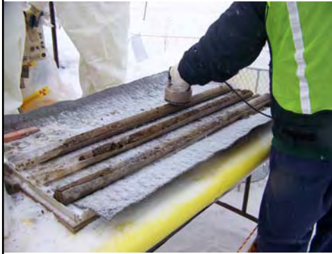
A rad tech surveys the core boring to check for Sr-90 contamination
