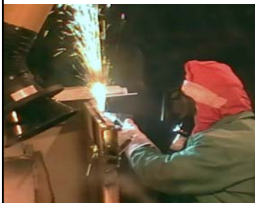
An operator uses plasma cutting technology to size-reduce contaminated components in the recently upgraded Container Size Reduction Facility
