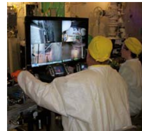
Operators at the controls for remote scabbling equipment
