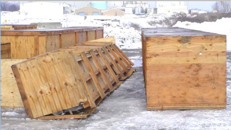
Box size: ~ 27 ft long, 3 ft wide, 3 ½ ft high Box weight: ~ 3,377 lbs
