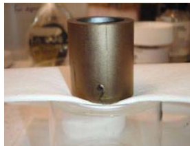
Lower Steam Jet Coupon After Acid Wash
