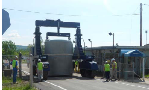
VCT Testing and Haul Road Verification was Conducted using an Empty Cask
