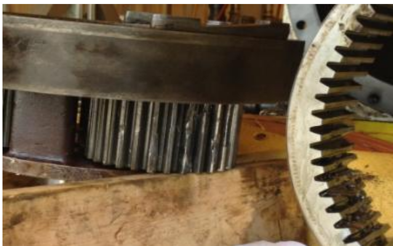
Damaged Planetary and Ring Gear
