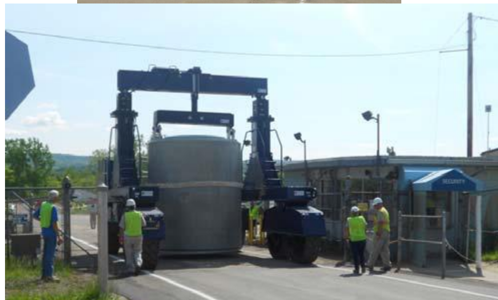
Vertical Cask Transporter (VCT) Testing and Haul Road Verification was Conducted using an Empty Cask
