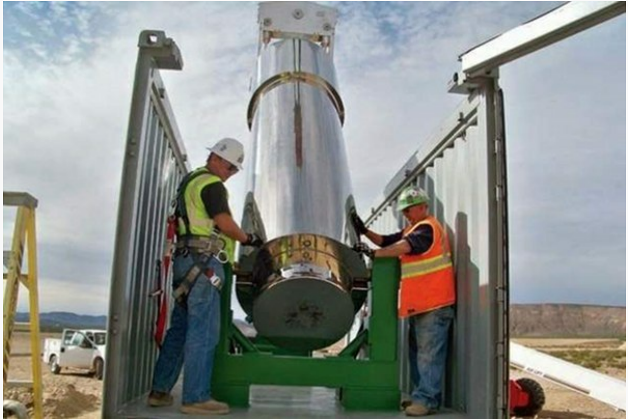
During training, workers removed a type of shipping cask that was expected to be used to transport 403 canisters of uranium-tainted waste from Oak Ridge National Laboratory to Nevada National Security Site northwest of Las Vegas. (File photo courtesy U.S. Department of Energy/Office of Environmental Management)
