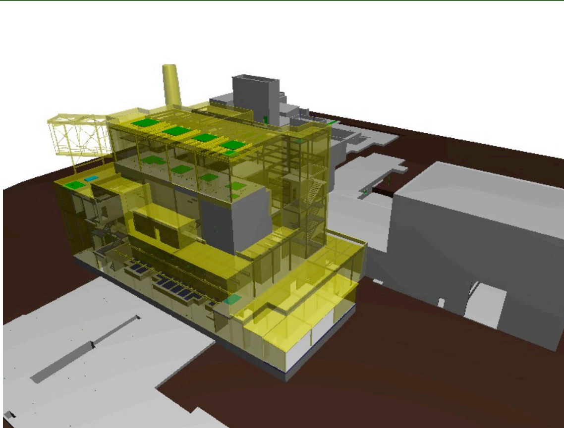
3-D Model of Main Plant Deconstruction (Completed areas in Yellow)
