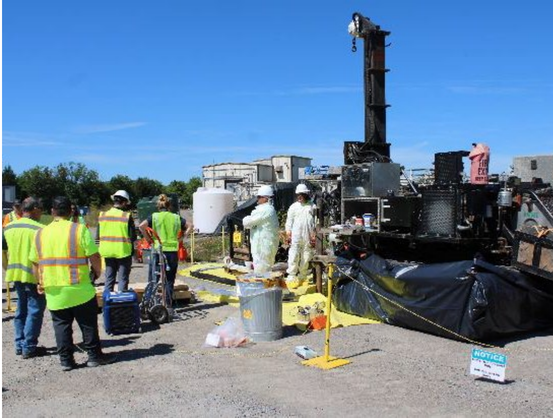
Core sampling operations
