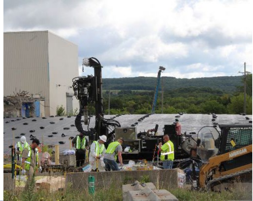
Core sampling operations
