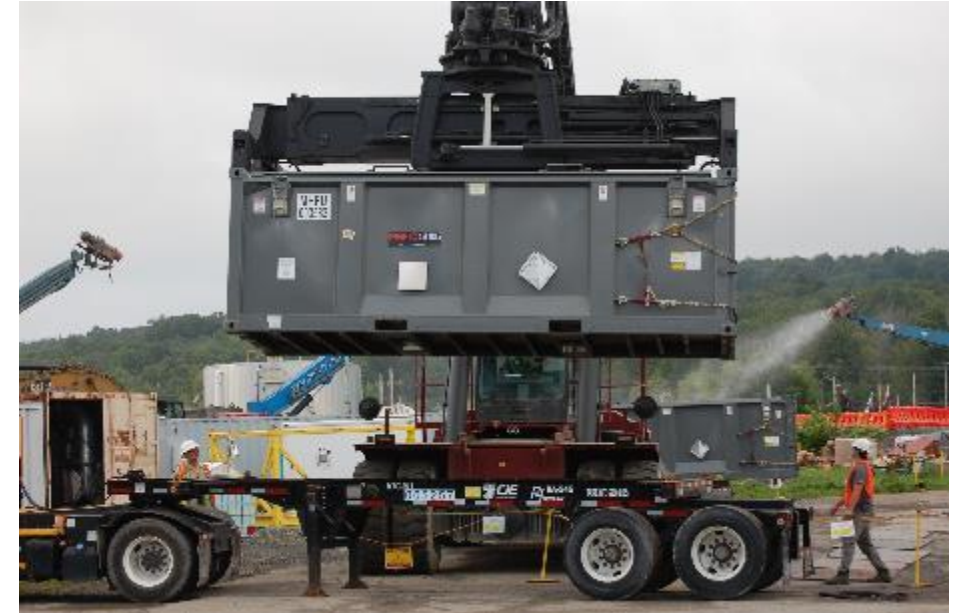
A reach-stacker places a full waste container onto a trailer for transport offsite
